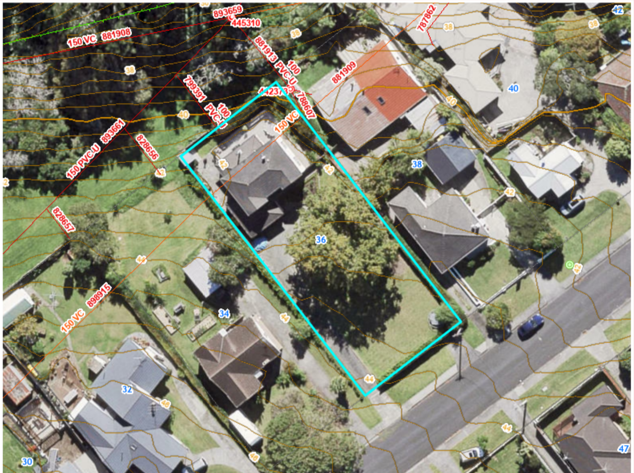
Figure 1: GIS Site aerial, showing stormwater (green) and wastewater connections (red), with contours in orange
